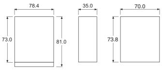
Enclosure for wall mounting to be used for thermostats, relay boxes, sensor enclosures
