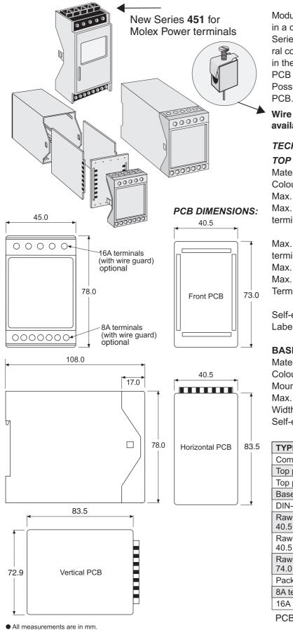
Module enclosure for M36 DIN-rail. To be used in a closed rack or installation box. Series 450 is, if requested, available in several colours and with customer specified holes in the front and base part. PCB and packing are available. Possibility for both vertical and horizontal PCB. Many PCB arrangements are possible.
