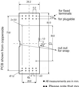
Module enclosure for M36 DIN-rail. Series 350 is, if requested, available in several colours and with customer specified holes in the front. Lid, PCB, customized label and packing is available.
